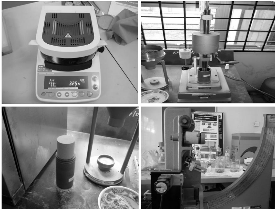
Fig.2: Equipment for foundry sand testing. Moisture analyser(top left), Ridsdale-Dietert metric standard rammer (top right), strip block (bottom left) and Ridsdale-Dietert universal sand strength (bottom right)
